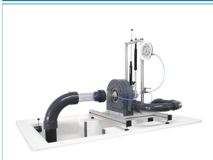
The TH 01.4 equipment simulates a small-scale installation with a Kaplan turbine.
